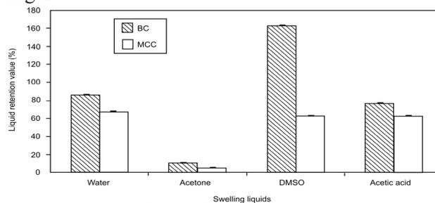
**Figure 4.** Swelling of bacterial cellulose and the commercial MCC in organic solvent.
